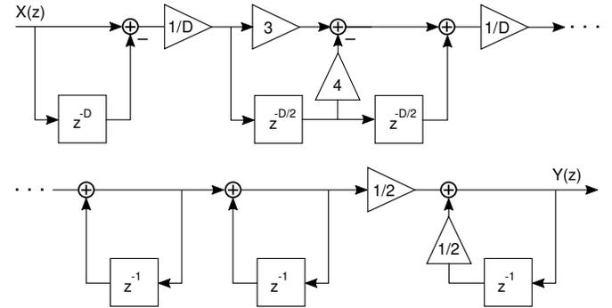
Fig. 9. Blockdiagram of the implemented BDF filter, where the delay  $D$  can be dynamically adapted.
