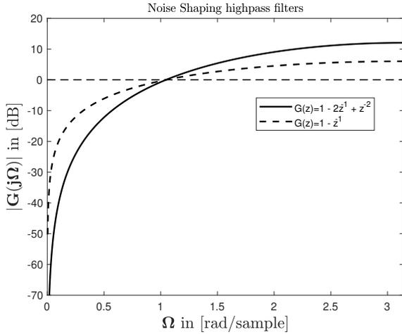
Fig. 5. Noise Shaping highpass filters.
