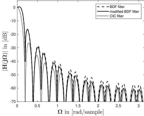
Fig. 3. Comparison of the presented filter types in second order form, where  $\Omega$  is the normalized frequency ( $\Omega = 2\pi f/f_s$ ) in radian per sample.
