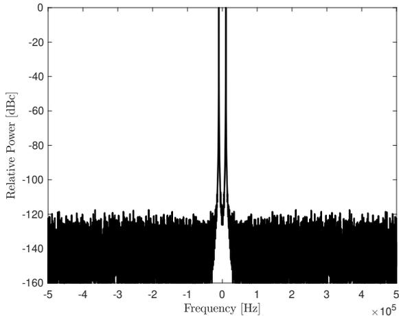
Fig. 8. 10kHz signal with a LUT width of 16 bits and no further processing (reference).
