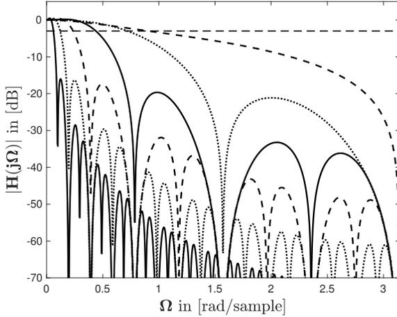
Fig. 4. BDF filters with delays from 64 down to 2.
