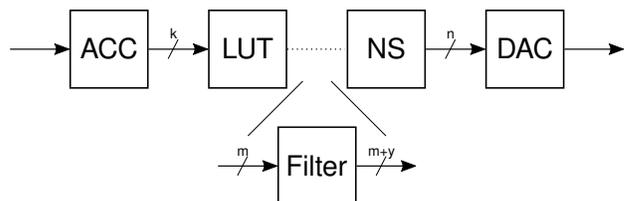
Fig. 2. Advanced DDS Structure
