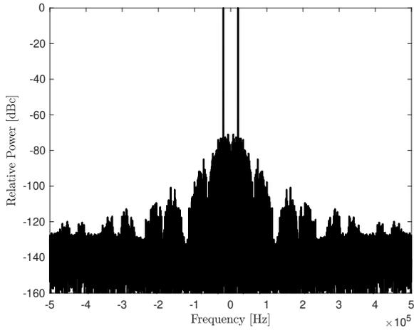
Fig. 7. 20kHz signal with a LUT width of 8 bits and a resulting bitwidth of 16 bits, achieved by BDF filtering and noise shaping.
