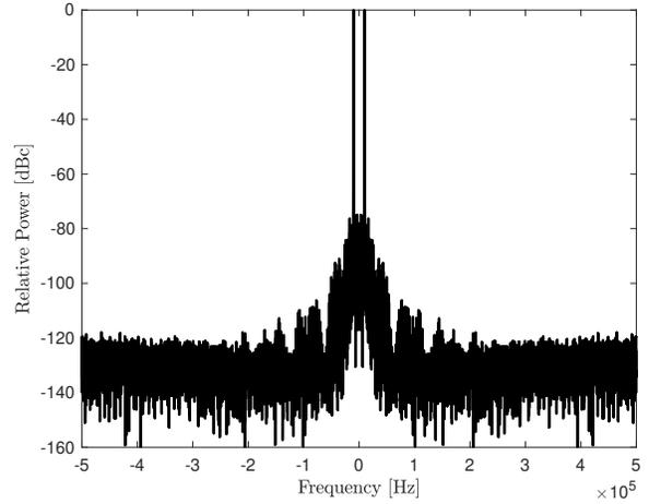
Fig. 6. 10kHz signal with a LUT width of 8 bits and a resulting bitwidth of 16 bits, achieved by BDF filtering and noise shaping.
